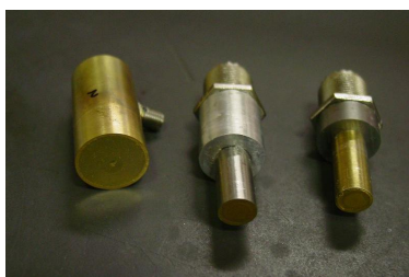
Figure 3. Three transducers developed in program: 75 MHz, 10 MHz and 15 MHz designs, from left to right. Electrical connection is achieved with an SMA connector for the 75 MHz device, and UHF connectors for the others.
